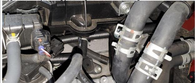
Page 1 of 2 1-27-23 **'05-'15 Tacoma; '05-'09 4runner, '07-'09 FJ Cruiser** (image #1 below) Set J&L Mounting bracket on front stud that holds engine cover on. Bracket will sit near the oil fill cap. Reinstall engine cover and reinstall nut back onto stud but do not tighten fully yet. Install J&L Oil separator to bracket with supplied M4 Screws.
